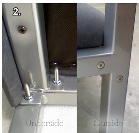
Step 2: On the underside of the Trados chair are 2 metal cross braces which support the seat. Using the Allen wrench (provided with the table) and a 7/16" wrench, remove the top bolt and nut from the same ends of both front and rear cross braces. This top bolt attaches the metal brace to the side brace. It is the bolt on the right in the picture shown at right. Make certain that this is the side you want to attach the connecting table to the chair.
