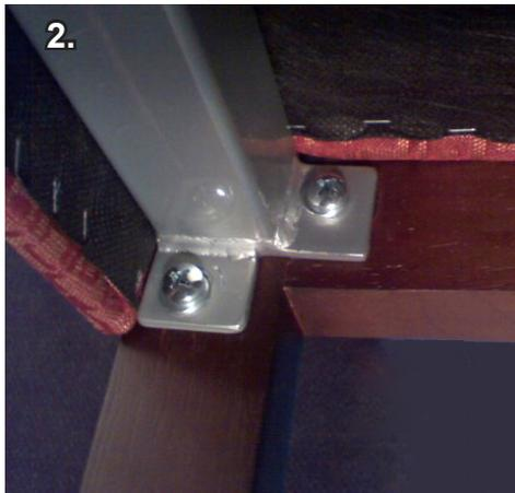
Step 2: On the underside of the Trados chair are 2 metal cross braces which support the seat. Using your phillips screwdriver, remove the top bolt from the same ends of both front and rear cross braces. This top bolt attaches the metal brace to the wooden side brace and is the bolt on the right in the picture shown at right. Make certain that this is the side you want to attach the connecting table to the chair.
